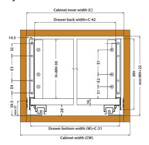
Note: Hole pattern printed represents our prototype and there are more options. It might have been altered according to our customer's needs. Dimensions in mm
