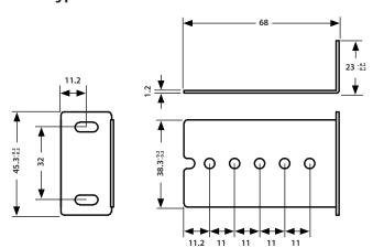
Note: Hole pattern printed represents our prototype and there are more options. It might have been altered according to our customer's needs. Dimensions in mm
